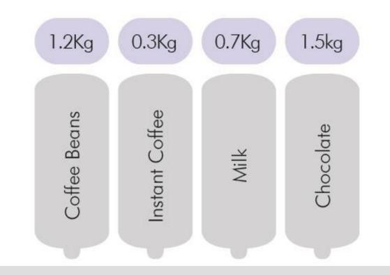
Designed throughput is 160 drinks before cleaning, emptying or reloading is required
